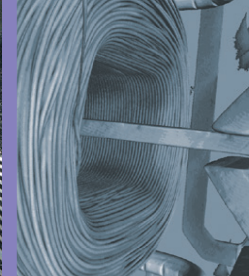
CT of a relay coil
